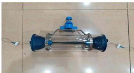
Gambar 3. 5 Alat *Water Point Sampler*
