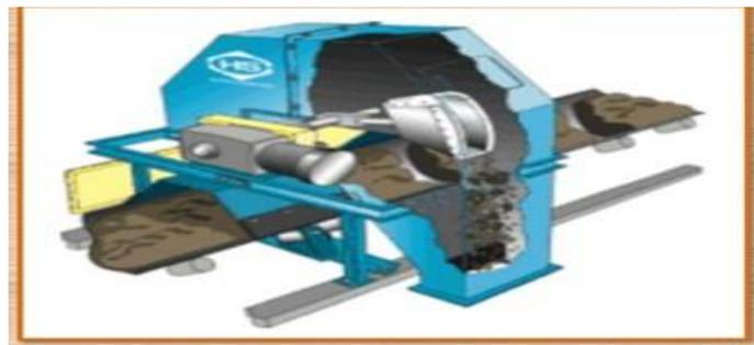
Gambar 3. 14 alat *sample cutter*
