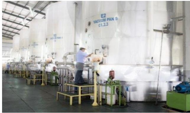
Gambar 3.10 Vaccum Pan Sumber PT Sugar Labinta
