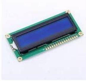
Gambar 2.3 LCD (*Liquid Crystal Display*)
