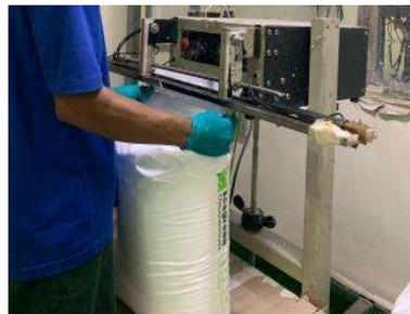
**Gambar 3. 53** Proses *Laminating*
