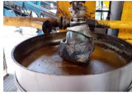
**Gambar 3. 20** *Vibrating Oil Screen*
