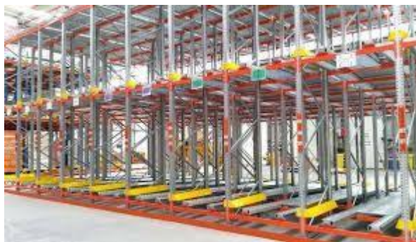
Gambar 2.7 Dynamic Storage Racking System
