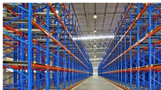
Gambar 2.1 Selective Pallet Racking
