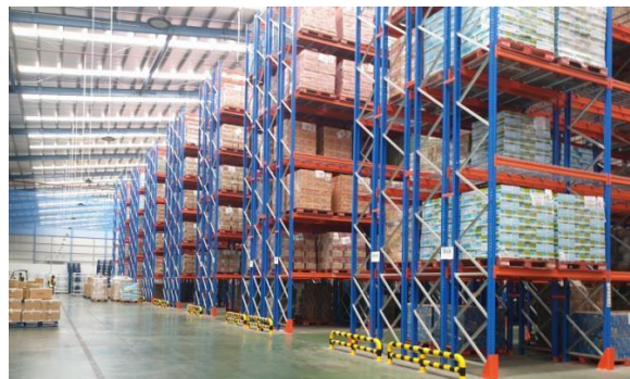
Gambar 2.2 Double Deep Racking
