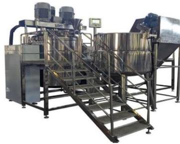
**Gambar 3.4** *Tank Homogenizer*
